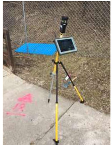
Part of the robotic total station being used for layout. The equipment utilizes GPS and computer programming to accurately lay out desired points.
